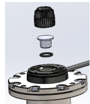
Pressure Test Cap Installation
