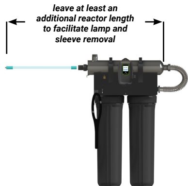
Figure 3. Lamp Removal Spacing
