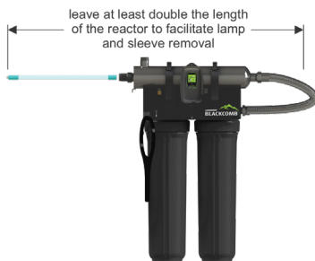
Figure 3. Lamp Removal Spacing
