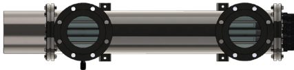
Figure 5b: Alternate orientation. Ensure sensor is on the bottom and chamber is vented
