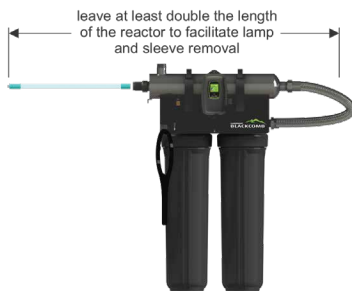
Figure 3. Lamp Removal Spacing
