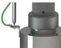
Figure 11. Ground Screw Connection
