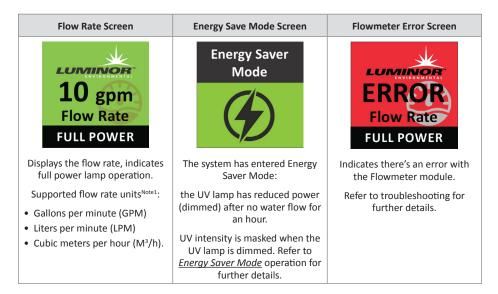
Note 1: The UV system units are set using the programmer. If a user wishes to have the flow units changed, they need to contact their plumber/dealer/distributer. Default is GPM.
