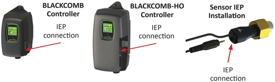
The Remote Alarm module comes with both a male and female IEP connection (Infinite Expandability Port). To initiate the module simply plug the male plug into the IEP on the Standard or High Output controller, or into any other BLACKCOMB module that contains an IEP (sensor, 4-20 mA module, solenoid module, etc.) and then restart the system.
