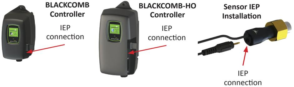
The UV Concierge module comes with both a male and female IEP connection (Infinite Expandability Port). To initiate the module simply plug the male plug into the IEP on the Standard or High Output controller, or into any other BLACKCOMB module that contains an IEP (sensor, 4-20 mA module, solenoid module, etc.), plug in the included power adapter to the wall and your UV Concierge module, and then restart the UV system.
