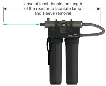
Figure 3. Lamp Removal Spacing
